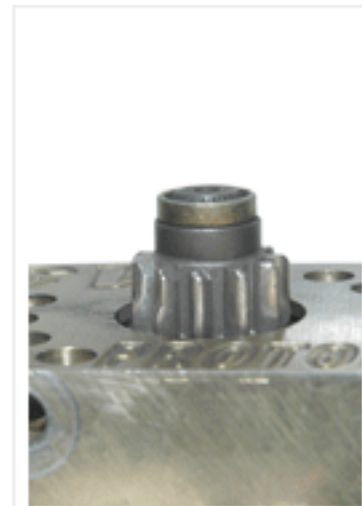
A Worn & Broken Gear Teeth (side)
